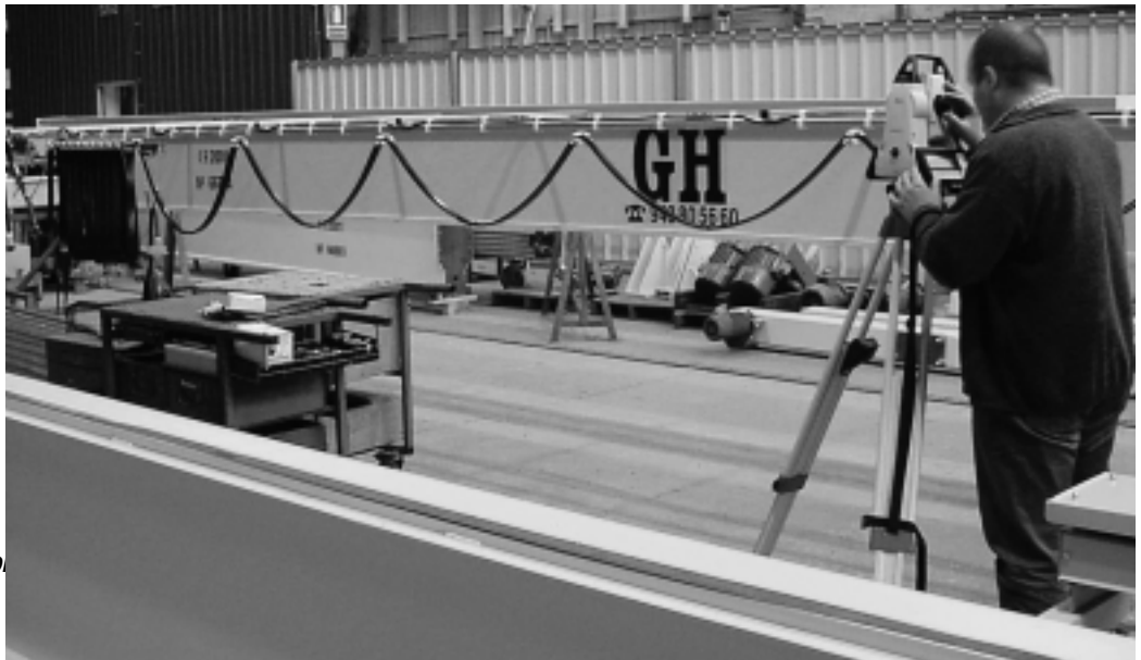
Large Scale CMM for dimensional checks on distances and angles of crane parts and railbeds
